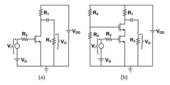
$$\begin{split} V_{DD} = 24V, V_G = 3V, R_1 = 5k\Omega, R_2 = 1k\Omega, R_3 = 20k\Omega, R_4 = 7k\Omega, R_5 = 5k\Omega \\ V_T = 1V, W/L = 60, K = 20\mu\text{A}/V^2 \end{split}$$
