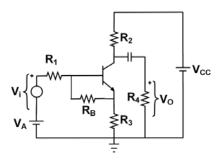
$\beta_f = 200, V_{CC} = 12V, V_A = 10V, R_B = 2k\Omega, R_1 = 15k\Omega, R_2 = 1k\Omega, R_3 = 0.5k\Omega, R_4 = 5k\Omega$
