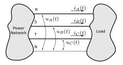
$$\begin{array}{lll} u_{AN}(t) &=& U_{\rm P}\sqrt{2}{\rm cos}\left(\omega t\right) \\ u_{BN}(t) &=& U_{\rm P}\sqrt{2}{\rm cos}\left(\omega t-\frac{2\pi}{3}\right) \\ u_{CN}(t) &=& U_{\rm P}\sqrt{2}{\rm cos}\left(\omega t+\frac{2\pi}{3}\right) \end{array}$$
