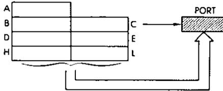
*Timing:*              3 M cycles; 12 T states; 6 usec @ 2 MHz
