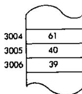
**PUSH qq** Push register pair onto stack.
