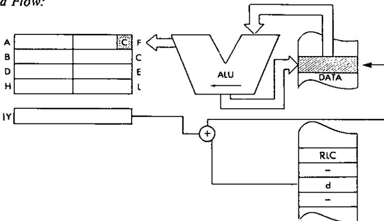
*Timing:* 6 M cycles; 23 T states; 11.5 usec @ 2 MHz
