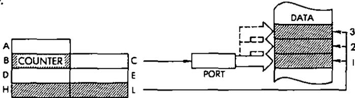
*Timing:*                               $B = 0$ : 4 M cycles; 16 T states; 8 usec @ 2 MHz.
