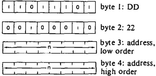
*Description:* The contents of the low order of the IX register are loaded into the memory location addressed by the contents of the memory location immediately following the opcode. The contents of the high order of the IX register are loaded into the memory location immediately following the one loaded from the low order. The low order of the nn address occurs immediately after the op code.
