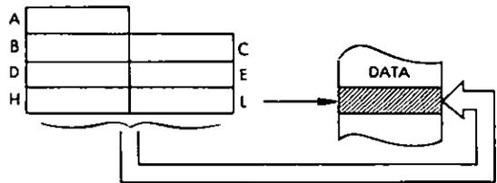
*Timing:* 2 M cycles; 7 T states; 3.5 usec @ 2 MHz
