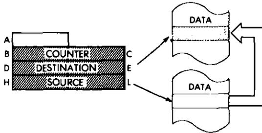
*Timing:*                      4 M cycles; 16 T states; 8 usec @ 2 MHz
