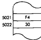
**LD dd, nn** Load register pair dd with immediate data nn.
