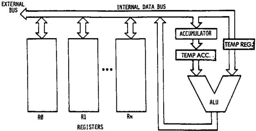
Fig. 2.13: Two Buffers Are Required (Temp Registers)
