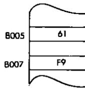
**LD (IX + d), n** Load indexed addressed memory location (IX + d) with immediate data n.
