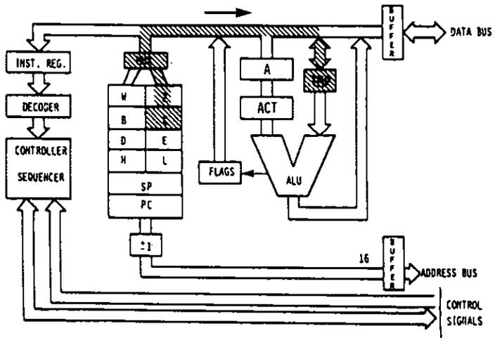
**Fig. 2.21: The Contents of C Are Deposited into TMP**
