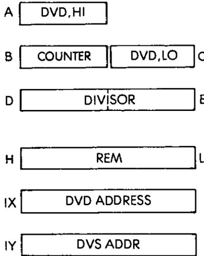
**Fig. 3.34: Non-Restoring Division—The Registers**
