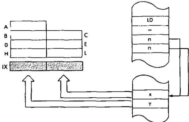
*Timing:* 6 M cycles; 20 T states; 10 usec @ 2 MHz
