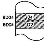
**LD A, (BC)** Load accumulator from the memory location indirectly addressed by the BC register pair.
