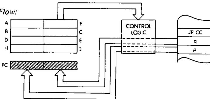
*Timing:* 3 M cycles; 10 T states; 5 usec @ 2 MHz
