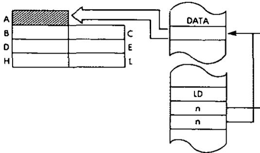
*Timing:* 4 M cycles; 13 T states; 6.5 usec @ 2 MHz
