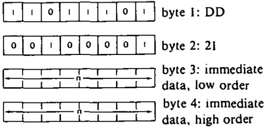
*Description:* The contents of the memory locations immediately following the opcode are loaded into the IX register. The low order byte occurs immediately after the opcode.
