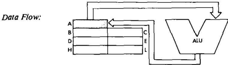
*Timing:*                      2 M cycles; 8 T states; 4 usec @ 2 MHz
