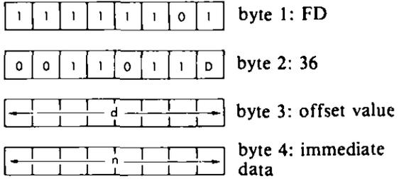
*Description:* The contents of the memory location immediately following the offset are transferred into the memory location addressed by the contents of the index register plus the given offset value.
