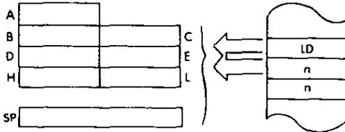
*Timing:* 3 M cycles; 10 T states; 5 usec @ 2 MHz
