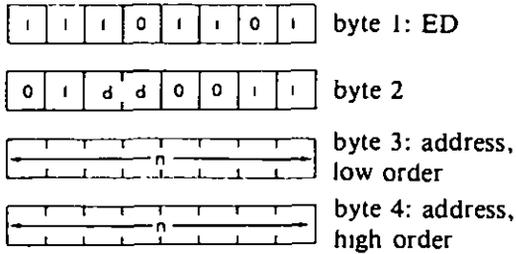
*Descriptions:* The contents of the low order of the specified register pair are loaded into the memory location addressed by the memory locations immediately following the opcode. The contents of the high order of the register pair are loaded into the memory location immediately following the one loaded from the low order. The low order of the nn address occurs immediately after the opcode. dd may be any of:
