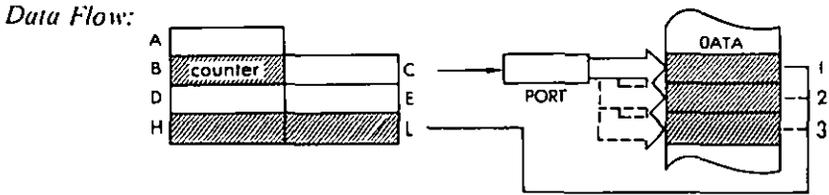
*Timing:*                               $B = 0$ : 4 M cycles; 16 T states; 8 used @ 2 MHz.
