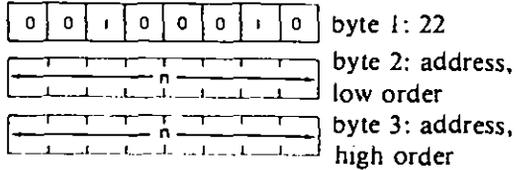
*Description:* The contents of the L register are loaded into the memory location addressed by the memory locations immediately following the opcode. The contents of the H register are loaded into the memory location immediately following the location loaded from the L register. The low order of the nn address occurs immediately after the opcode.
