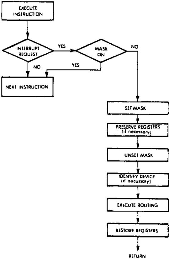
Fig. 6.34: Interrupt Logic
