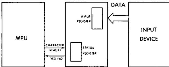
**Fig. 6.8a: Handshaking (Input)**
