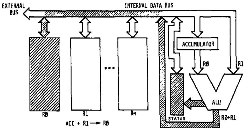
Fig. 2.11: Result Is Generated and Goes into R0
