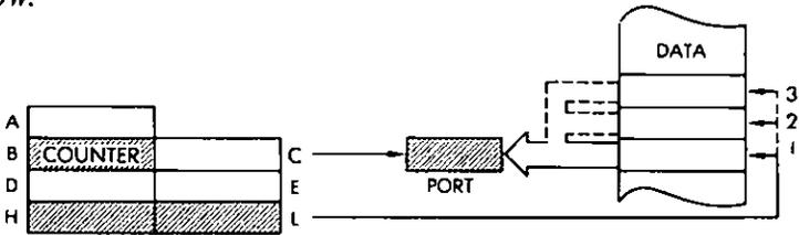
*Timing:*                       $B = 0$ : 4 M cycles; 16 T states; 8 usec @ 2 MHz.
