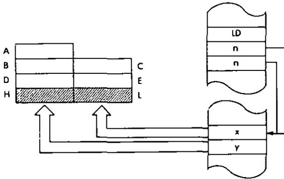
*Timing:* 5 M cycles, 16 T states; 8 usec @ 2 MHz
