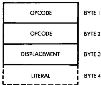
Fig. 5.5: Indexed Addressing Has 2-byte Opcode
