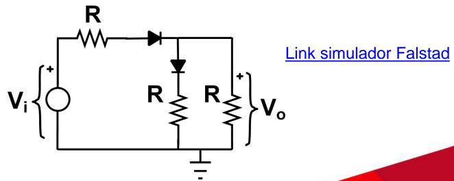
$V_{\gamma} = 0.7V$ ,  $R = 800\Omega$ ,  $|V_R| = 50V$ ,  $I_{max} = 25mA$
