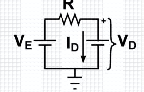
$R = 1.2k\Omega, V_{\gamma} = 0.65V, |V_Z| = 5.6V, I_{MAX} = 25mA, I_{Z,MIN} = 5mA, P_{Z,MAX} = 168mW$
