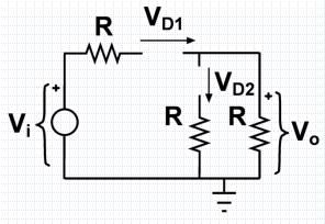
$V_{\gamma} = 0.7V$ ,  $R = 800\Omega$ ,  $|V_R| = 50V$ ,  $I_{max} = 25mA$
