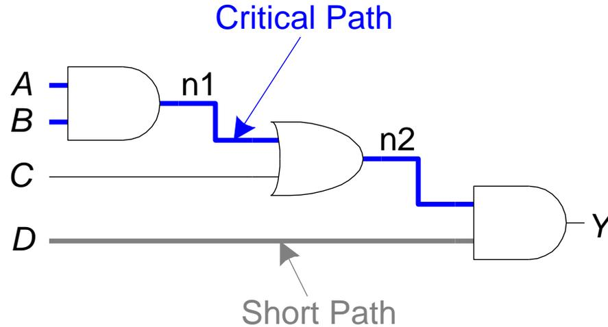
**Ruta crítica:**  $t_{pd} = 2t_{pd\_AND} + t_{pd\_OR}$
