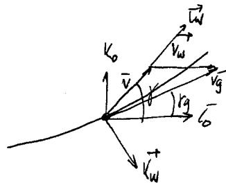
$$\frac{dx_0}{dt} = v_g \text{sen} \cdot \vec{e}_g = V_{G0} \cdot \text{sen} \cdot \vec{e}_g + v_{w0} + k_w t ; \boxed{x_0 = \int_{x_0}^t (V_{G0} \cdot \text{sen} \left( \frac{V}{R} t \right) + v_{w0} + k_w t) dt = R \text{sen} \frac{Vt}{R} + v_{w0} t + \frac{k_w t^2}{2}}$$
