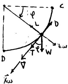
$$\vec{v} = \dot{\varphi} R_2 \vec{i}_w \quad \ddot{\varphi} R_2 = V \\ \ddot{a} = -\dot{\varphi}^2 R_2 \vec{k}_w$$
