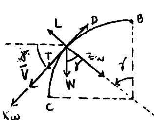
$$\begin{aligned} \vec{V} &= R \dot{\gamma} \vec{i}_{\omega} \rightarrow \dot{\gamma} = \frac{V}{R} = \text{cte} \\ \vec{a} &= \dot{\gamma}^2 R \vec{k}_{\omega} \\ E.F. &= m \cdot \vec{a} \quad \left\{ \begin{array}{l} \vec{i}_{\omega}: T - D + W \cdot \sin \gamma = 0 \quad (1) \\ \vec{k}_{\omega}: -L + W \cos \gamma = m \dot{\gamma}^2 R = \frac{V^2}{R} W \quad (2) \end{array} \right. \end{aligned}$$
