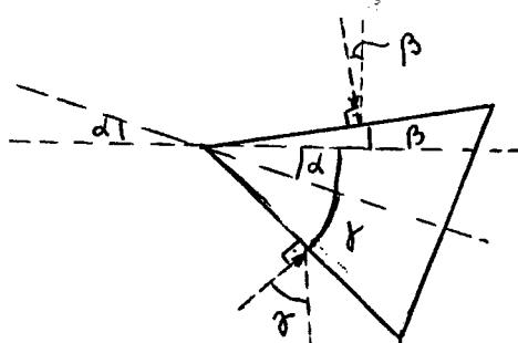
$$\begin{aligned} \beta &= \frac{\delta}{2} - \alpha \\ \gamma &= \frac{\delta}{2} + \alpha \end{aligned}$$
