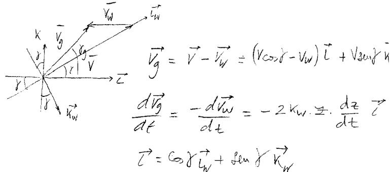
$$\frac{dV_g}{dt} = \vec{v} - \vec{V}_w = (V \cos \varphi - V_w) \vec{i} + V \sin \varphi \vec{k}$$
