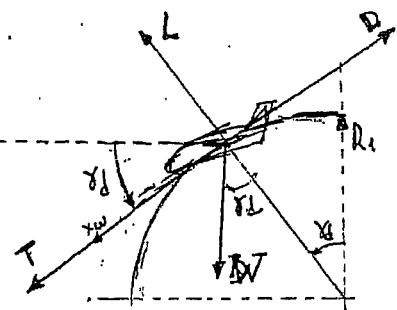
$$\gamma_d = \frac{V}{R_1} \rightarrow \gamma_d = \frac{V \cdot t}{R_1}$$
