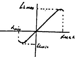
$$\alpha_{min} < \alpha = C_{L0} + C_{Lad} < \alpha_{max}$$
