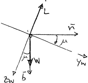
$$\begin{cases} \bar{b} = \cos \mu \bar{k}_w + \sin \mu \bar{j}_w \\ \bar{n} = \cos \mu \bar{j}_w - \sin \mu \bar{k}_w \end{cases}$$
