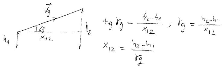
$$\tan \theta_g = \frac{h_2 - h_1}{x_{12}}, \quad \theta_g = \frac{h_2 - h_1}{x_{12}}$$
