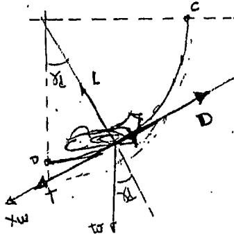
$$\bullet \gamma_d = \frac{\pi}{2} - \frac{V}{R_2} t \rightarrow \dot{\gamma}_d = -\frac{V}{R_2}$$
