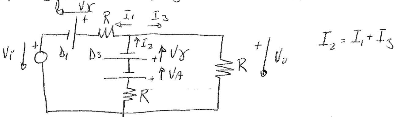
$$I_1 : V_c + V_\gamma + I_1 R = V_o \Rightarrow I_1 = \frac{V_o - V_c - V_\gamma}{R}$$
