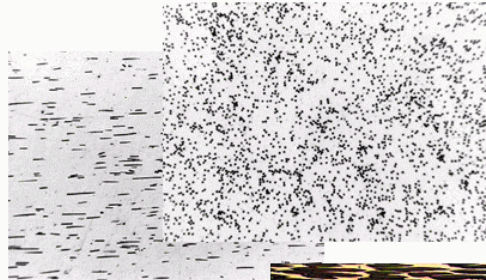
Al matrix / short high modulus carbon fibres composite made by hot extrusion of powdered mixture
