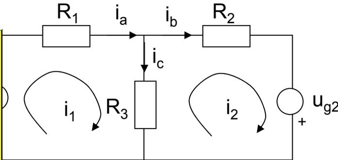
$$\left. \begin{aligned} -u_{g1} + i_1 R_1 + (i_1 - i_2) R_3 &= 0 \\ -u_{g2} + i_2 R_2 + (i_2 - i_1) R_3 &= 0 \end{aligned} \right\}$$
