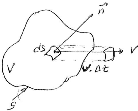
Moving control volume used for the physical interpretation of the divergence of velocity at some instant time.
