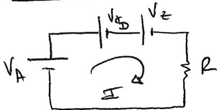
$$I = \frac{V_A - V_Z - V_{\gamma_D}}{R}$$
