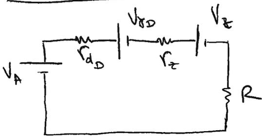
$$I = \frac{V_A - V_{\gamma_D} - V_Z}{R + r_{d_D} + r_{\gamma_Z}}$$
