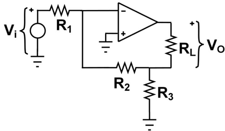
$$V_{CC} = 12 \text{ V}, V_{EE} = -12 \text{ V}, R_1 = 4 \text{ k}\Omega, R_2 = 10 \text{ k}\Omega, R_3 = 2 \text{ k}\Omega, R_L = 7 \text{ k}\Omega$$
