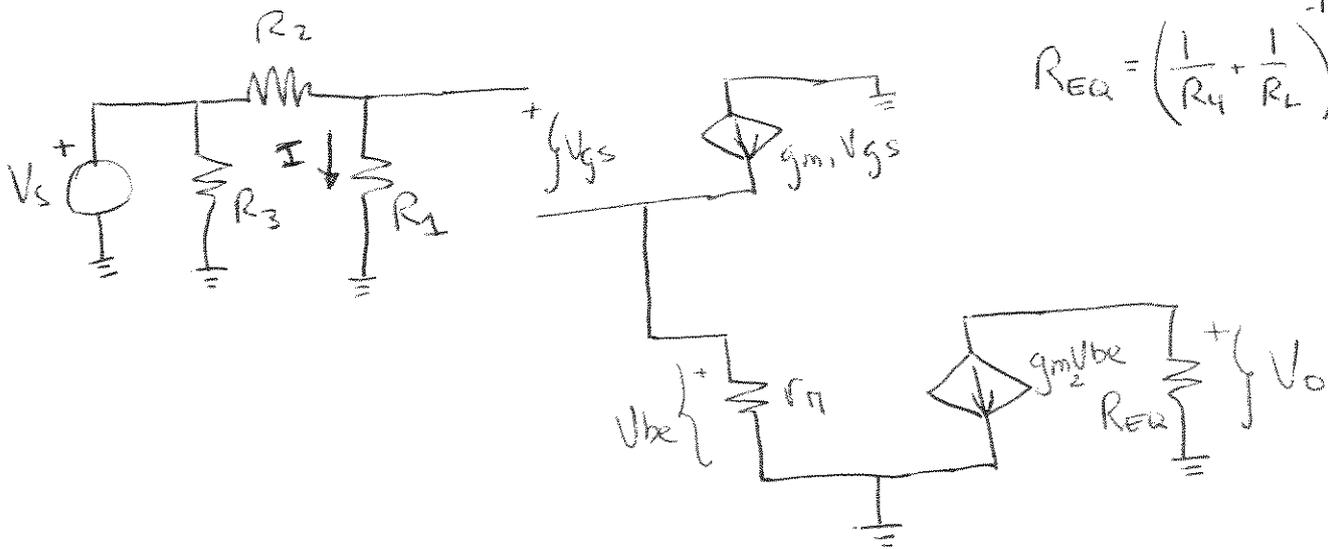
$$R_{EQ} = \left( \frac{1}{R_4} + \frac{1}{R_L} \right)^{-1} = 857 \Omega$$
