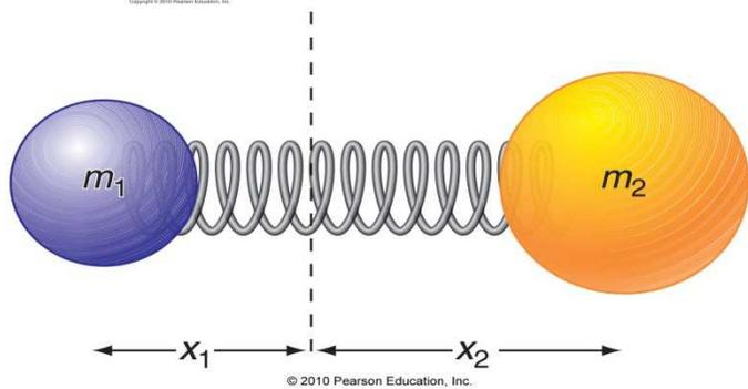
$$F = \mu a = \mu \frac{d^2x}{dt^2} \longrightarrow \mu \frac{d^2x}{dt^2} + kx = 0$$
