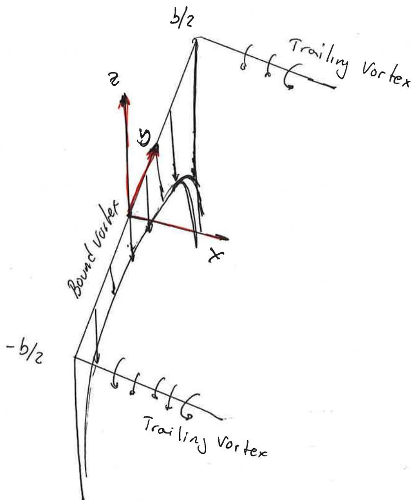
The two trailing vortices both contribute to induced velocity along the bound vortex, and these contributions are in the downward direction. The direction is negative ( $w$ ) ( $z$  direction). The velocity at any point  $y$  along the bound vortex induced by the trailing semi-infinite vortices is given by  $V = \frac{\Gamma}{4\pi h}$ .
