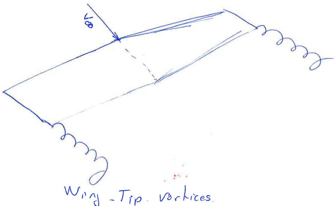
The tendency for the flow to "turn" around the wing tips has another important effect on the aerodynamics of the wing. This flow establishes a circulatory motion that trails downstream of the wing; that is, a trailing vortex is created at each wing tip. Tip vortices are essentially weak "tornadoes" that trail downstream of the finite wing. These wing-tip vortices downstream of the wing induce a small downward component of air velocity in the neighborhood of the wing itself.
