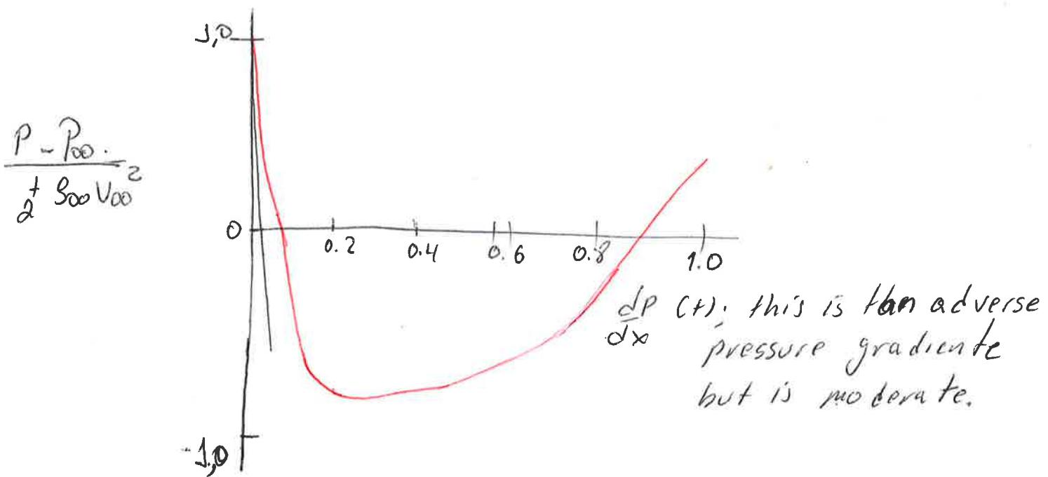
Pressure distribution over the top for attached flow over an airfoil.
