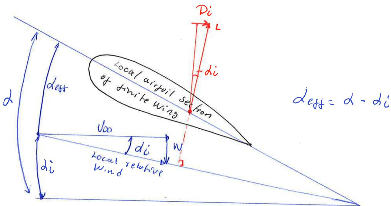
1. The angle of attack actually seen by the local airfoil section is the angle between the chord line and the local relative wind.  $\alpha_{\text{eff}}$ , effective angle of attack.
