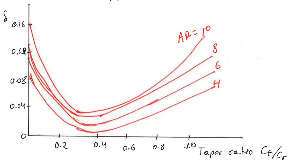
The variation of  $\delta$  as function of taper ratio for wings of different A.R. with this graph a tapered wing can be designed with an induced drag coefficient reasonably close to the minimum value. The manufacture is considerable easier to manufacture than elliptic planform.
