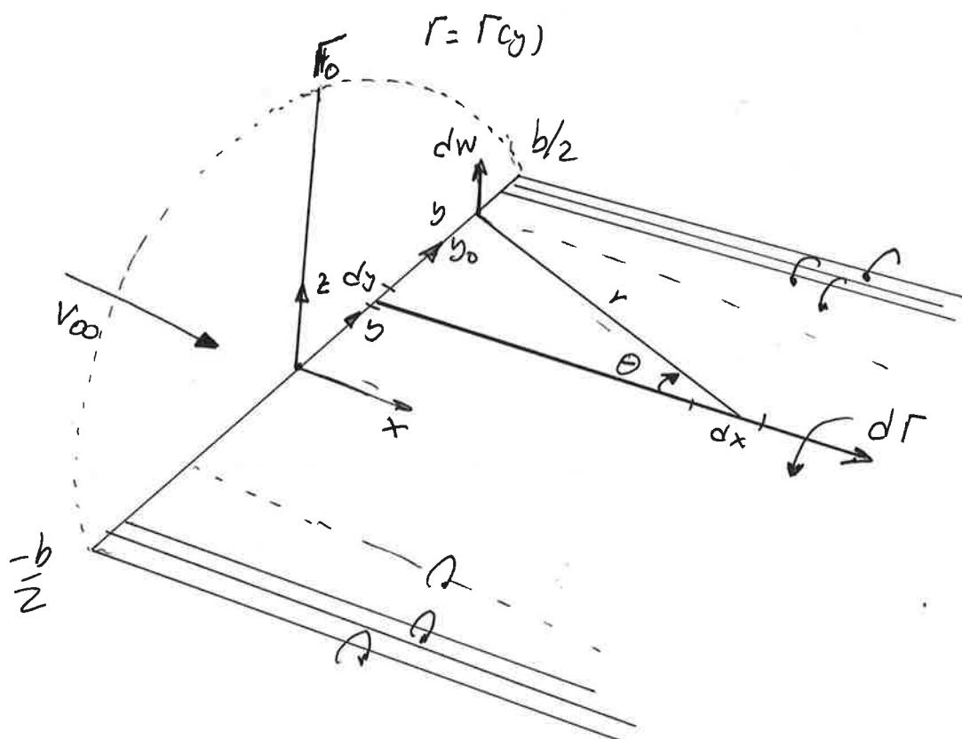
The value of the circulations at origin is  $\Gamma_0$ . The finite number of trailing vortices have become a continuous vortex sheet trailing downstream of the lifting line. This vortex sheet is parallel to the direction of  $V_{\infty}$ . The total strength of the sheet integrated across the span of the wing is zero, because it consists of pairs of trailing vortices of equal strength but in opposite direction.
