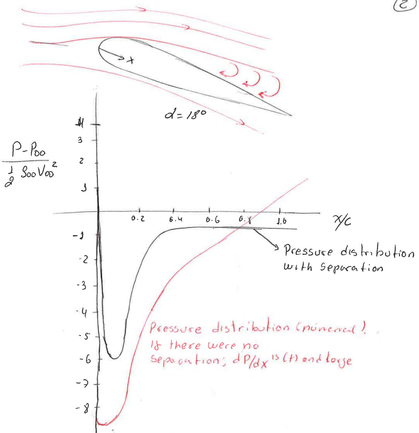
The adverse pressure gradient would be severe: that is,  $dP/dx$  would be large. In such case, the real viscous flow tends to separate from the surface.
