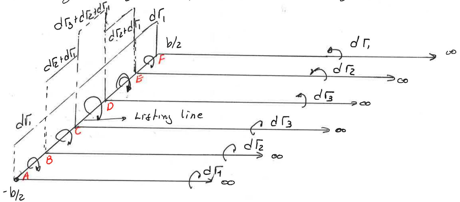
Let us extrapolate to the case where an infinite number of horseshoe vortices are superimposed along the lifting line, each with a vanishingly small strength  $d\Gamma$ .
