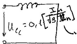
$$E_c - \frac{U_{cc,m}}{U_{u_1}} = \frac{\sqrt{3} \cdot I_{n1} \cdot Z_{cc}}{U_{u_1}} \Rightarrow Z_{cc} = E_c \frac{U_{u_1} \cdot U_{u_1}}{\sqrt{3} I_{n1} U_{u_1}} = E_c \frac{U_{u_1}^2}{S_1} = 0,1 \cdot \frac{(66 \cdot 10^3)^2}{10 \cdot 10^6} =$$
