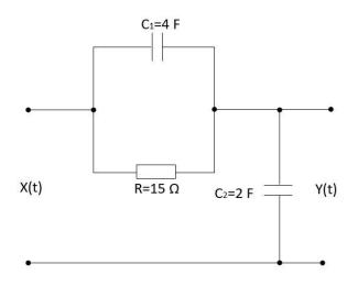
2.22 A white noise X(t) with  $R_{XX} = 4 \cdot 10^{-3} \cdot \delta(\tau)$  is filtered with the network of the figure below. Find the average power of the input and output of the system.
