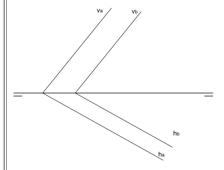
5. Consider an installation where two pipes (represented by lines r and s) must be connected by means of a third one. Find the minimum length of the third pipe and the points between which it has to be installed.
