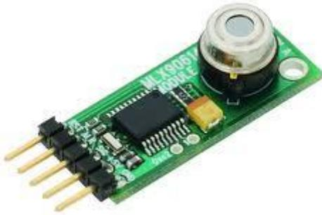
MLX90614 Infrared Thermometer Module
