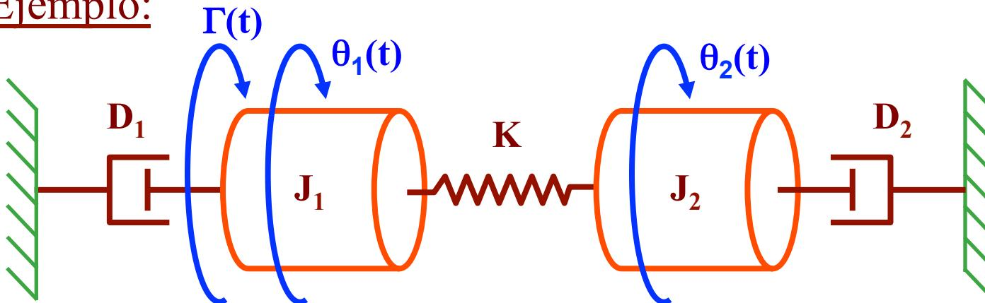
$$\begin{aligned} \sum \text{Imped}_1 \cdot \theta_1(s) - \sum \text{Imped}_{1-2} \cdot \theta_2(s) &= \sum \text{Pares}_1 \\ - \sum \text{Imped}_{2-1} \cdot \theta_1(s) + \sum \text{Imped}_2 \cdot \theta_2(s) &= \sum \text{Pares}_2 \end{aligned}$$
