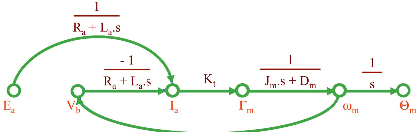
$$\left. \begin{aligned} T_1 &= \frac{1}{R_a + L_a \cdot s} K_t \frac{1}{J_m \cdot s + D_m} \frac{1}{s} \\ B_{11} &= \frac{-1}{R_a + L_a \cdot s} K_t \frac{1}{J_m \cdot s + D_m} K_b \\ \Delta &= 1 - B_{11} \end{aligned} \right\} \quad \Delta_1 = 1$$
