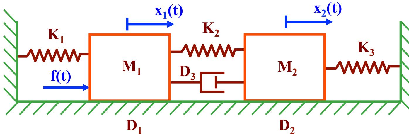
$$\sum \text{Imped}_1.X_1(s) - \sum \text{Imped}_{1-2}.X_2(s) = \sum \text{Fuerzas}_1$$
