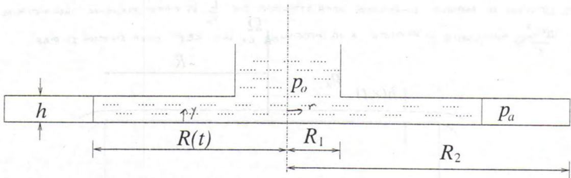
$$0 = -\frac{\partial P}{\partial r} + \mu \frac{\partial^2 v}{\partial y^2} \rightarrow v = -\frac{1}{2\mu} \frac{\partial P}{\partial r} y(h-y), \quad \int_0^h v dy = -\frac{h^3}{12\mu} \frac{\partial P}{\partial r}$$
