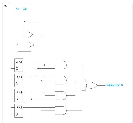
This shows the lowermost bit of each word. This schematic is repeated 7 more times for the remaining seven bits. Note that there are no connections for D and C flip-flop inputs because datapath figures do not specify how instruction memory is written.
