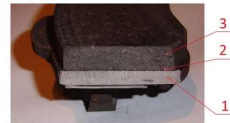
Figure 2: Key brake pad components: 1- back plate, 2- underlayer, 3- friction material
