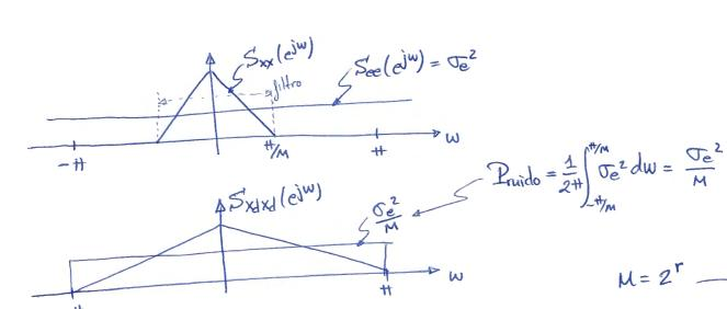
$$SNR(dB) = 10 \cdot log_{10} \left( \frac{Pseñal}{Pruido} \right) = 10 \cdot log_{10} \left( \frac{\nabla x^2}{\nabla_e^2} \cdot M \right) = SNR(dB) \left| \begin{array}{c} +3.01 \cdot r \\ \text{cuantiff} \\ \text{directa} \end{array} \right|$$
