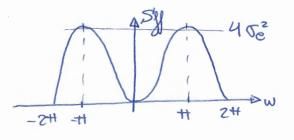
$$\text{CI } Sgg(e^{iw}) = Sg(e^{iw}) \cdot |H(e^{iw})|^2 = |Sg(e^{iw})| |w| \leq w_c$$
