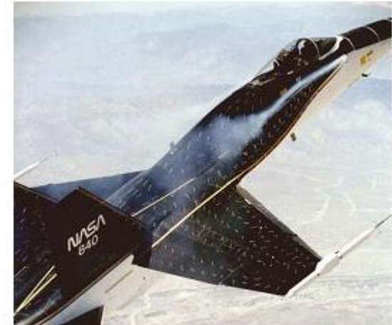
Figure 1. NASA F-18 High Angle of Attack Research Vehicle (HARV). Photo Courtesy of NASA Dryden.
