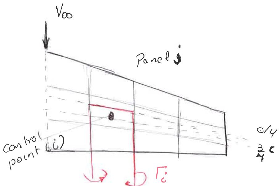
Bound vortex is located at panel  $\frac{1}{4}$  chord position with two trailing vortex lines shed from each end.
