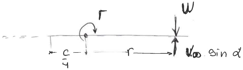
Planar airfoil section indicating location of control point where flow is parallel to the surface?
