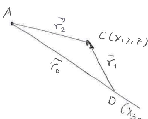
Induced velocity by the filament that extends from  $A$  to  $\infty$ .
