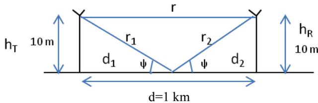
$$\psi = \text{atan} \left[ \frac{h_T}{d_1} \right] = \text{atan} \left[ \frac{h_R}{d_2} \right] \quad d = d_1 + d_2 = 10 \text{ km} \quad d_1 = d_2 = 500 \text{ m}$$
