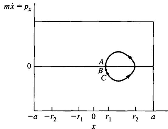
**FIGURE 11.5** A  $p_x x$  Poincaré section for the Kepler problem with the solid curve on the right tracing out the orbit generated by points  $A, B, C, \dots$  of the precessing ellipse of Fig. 11.4. Points  $A', B', C'$  are not shown but are located at negative values of  $x$ .
