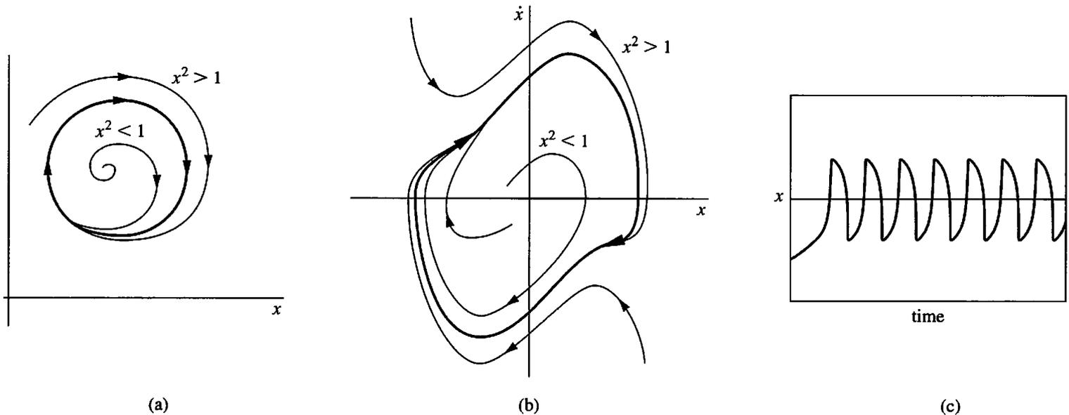
**FIGURE 11.3** Limit cycles (darkened curves) of the van der Pol equation in the  $\dot{x}$ ,  $x$  phase space showing (a) circular motion for a small damping coefficient  $\epsilon$ , and (b) distorted curve for large damping. Approaches to the limit cycles via orbits outside and inside them are shown. Part (c) sketches the distorted sine wave obtained for the case of appreciable damping (large  $\epsilon$ ).
