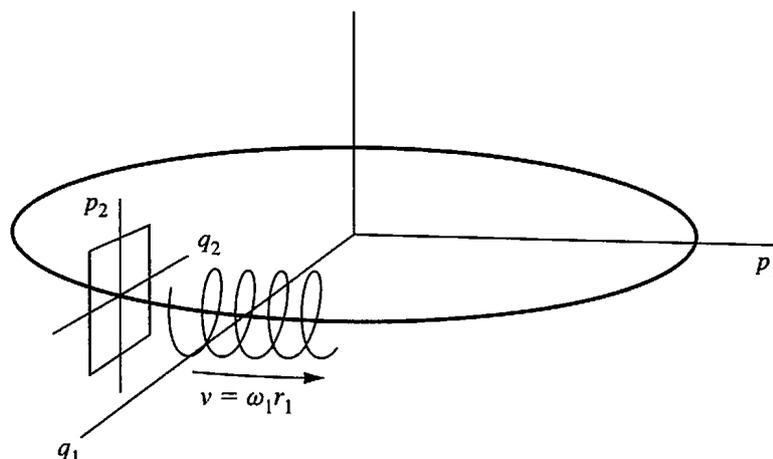
**FIGURE 11.2** Circular motions of a low-frequency ( $\omega_1$ ) harmonic oscillator in the horizontal  $p_1, q_1$  plane and of a high-frequency ( $\omega_2 > \omega_1$ ) harmonic oscillator in the uniformly moving  $p_2, q_2$  vertical plane. The oscillators are uncoupled, and the resultant spiraling motion of the second oscillator generates a torus, as shown.
