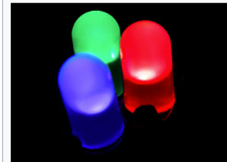
Blue, green, and red LEDs in 5 mm diffused case
