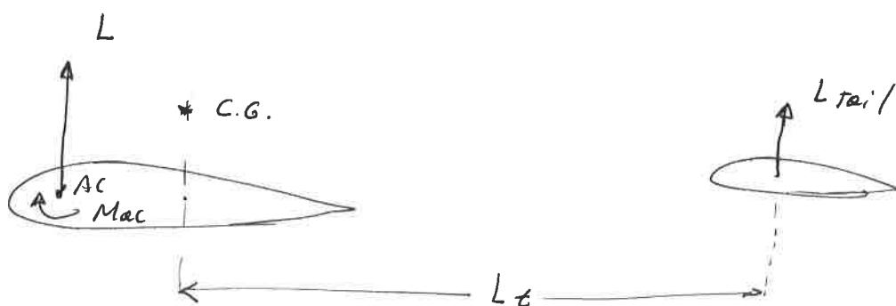
It is seen that the tail contributes a stabilizing moment when the wing-tail configuration is disturbed from equilibrium, and by a proper adjustment of the tail area and tail length Lt, this stabilizing moment can be made easily to outweigh the destabilizing effect of wing.
