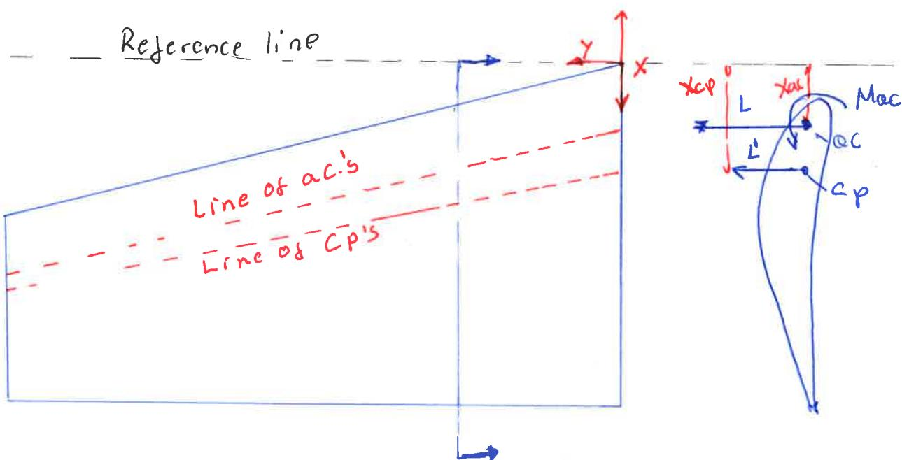
In this equation  $X_{ac}$  and  $M_{ac}$  are functions only of  $y$ ; since they are independent of the angle of attack, however,  $L'$  is a function of  $y$ , therefore of the sectional absolute angle of attack,  $\alpha_a$ . It follows that  $M_{ac}$  will be a function of  $\alpha_a$ , the absolute angle of attack of the wing and  $X_{cp}$  will be also be a function of  $\alpha_a$ .
