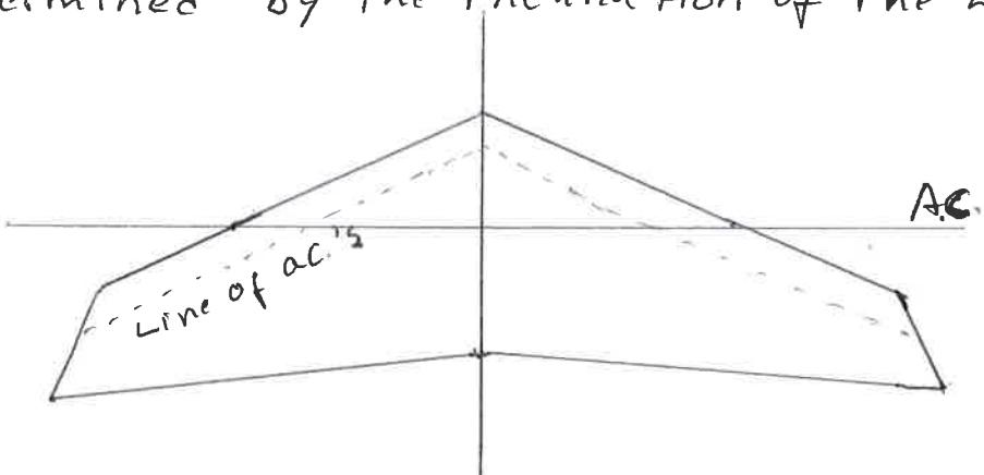
Presume that the wing is set at  $C_L = 0$  so that the lift acting at any section is basic lift, then if the wing is washed out at the tips, the lift acting on the outboard sections will be down, whereas the lift acting on the inboard section will be up. This consequence of the fact that the integral of the basic lift is zero. the basic lift thus distributed will cause a positive moment about the aerodynamic center.
