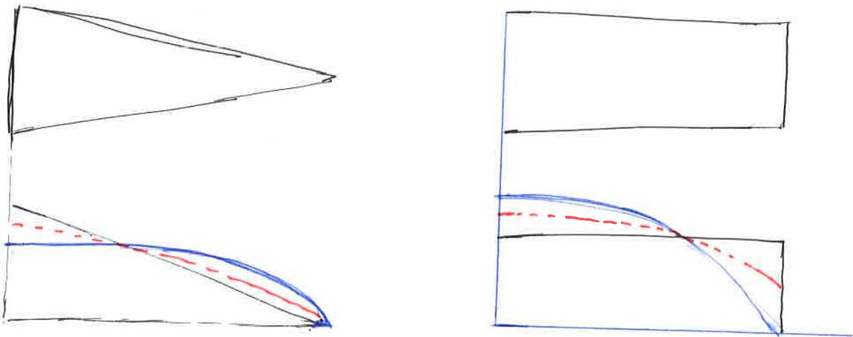
The red lines are drawn halfway between the actual chord and that for an ellipse of the same area and semi-span. We can observe that the effect of taper is to increase the load in the outboard portion above that which occurs if the additional lift were proportional to the chord.
