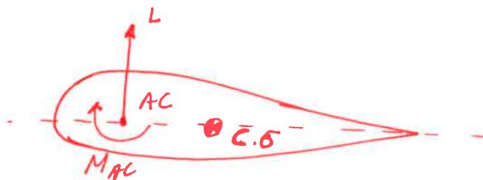
Wing cross section is shown with the load systems acting at aerodynamic center. Consider a wing as a rigid body, any unbalanced moments will cause it to rotate about its center of gravity.
