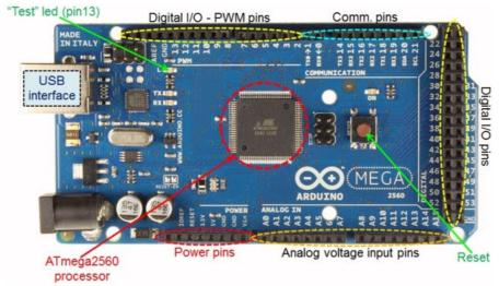
This **on-board LED is connected to <u>PORT B's bit 7</u>** in the Arduino Mega2560; the same bit is connected to Arduino's output pin 13 (so an external LED can be also connected). . Some words of warning: in older Arduino models, the on-board LED was traditionally connected to *PORT B's bit 5*, so check that for your Arduino model before using this LED.
