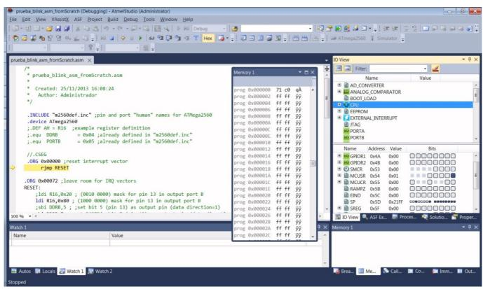
The "I/O View" panel appears at the right side of the window, showing the contents of the different parts of the Atmel processor (ports, CPU registers, etc.). Another window allows exploring the contents of the different memories: FLASH program memory, SRAM data memory (R0 to R32 are the 32 first positions of it), EEPROM memory.
