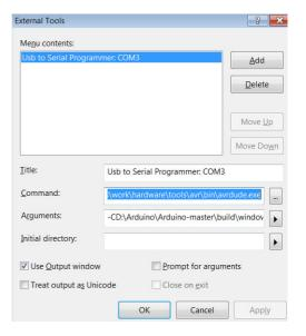
And that's all. You only need to do this once, from now on you can upload any program directly from the Tools menu; here a new entry with the name you gave to the tool will appear. By selecting it, your .hex program will be uploaded to the Arduino.
