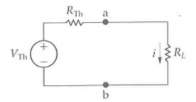
$$p = i^2 R_L = \left(\frac{V_{\text{Th}}}{R_{\text{Th}} + R_L}\right)^2 R_L$$
