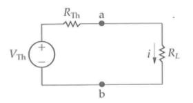
$$p = i^{2} R_{L} = \left(\frac{V_{\text{Th}}}{R_{\text{Th}} + R_{L}}\right)^{2} R_{L}$$
