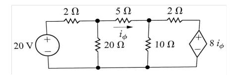
• If the **only element between two essential nodes is a voltage source**, the number of equations is reduced by one since the voltage source will impose the value of the node voltage between those essential nodes.
