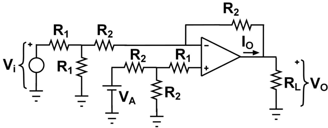
Datos:  $R_1 = 1 \text{ k}\Omega$ ,  $R_2 = 2 \text{ k}\Omega$ ,  $R_L = 1.2 \text{ k}\Omega$ ,  $V_A = 8\text{V}$ ,  $I_{o,\text{max}} = 25 \text{ mA}$
