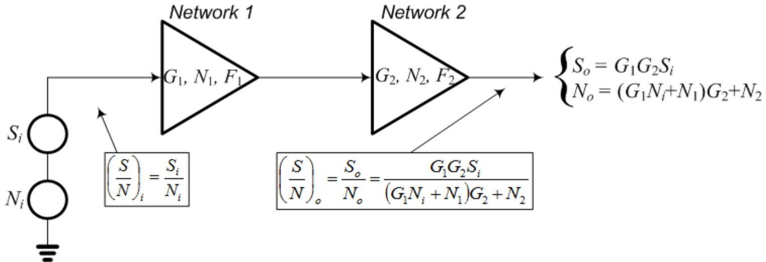
$$F_{comp} = \frac{(S/N)_i}{(S/N)_o} = \frac{S_i/N_i}{G_1 G_2 S_i / ((G_1 N_i + N_1) G_2 + N_2)} = \frac{G_1 N_i + N_1}{G_1 N_i} + \frac{N_2}{G_1 G_2 N_i} = \underbrace{\left(1 + \frac{N_1/G_1}{N_i}\right)}_{F_1} + \frac{1}{G_1} \underbrace{\left(\frac{N_2/G_2}{N_i}\right)}_{F_2 - 1} = F_1 + \frac{F_2 - 1}{G_1}$$
