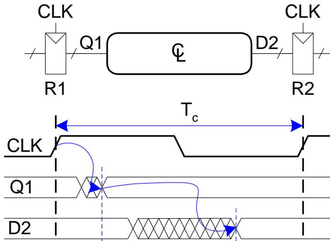
$$T_c \geq t_{pcq} + t_{pd} + t_{\text{setup}}$$
