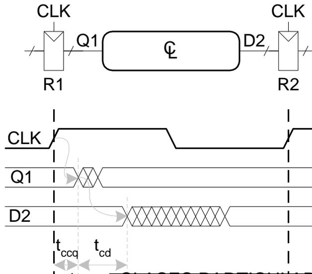
$$t_{\text{hold}} < t_{\text{ccq}} + t_{\text{cd}}$$
