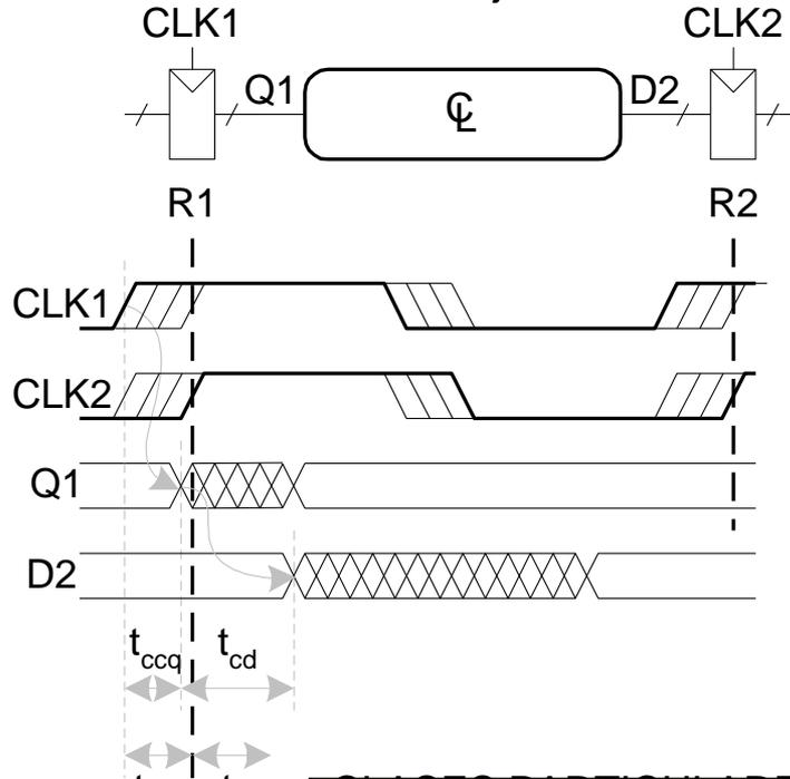
$$t_{ccq} + t_{cd} > t_{hold} + t_{skew}$$
