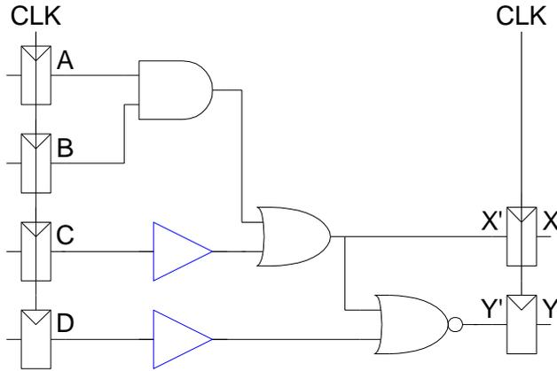
$$t_{pd} = 3 \times 35 \text{ ps} = 105 \text{ ps}$$
