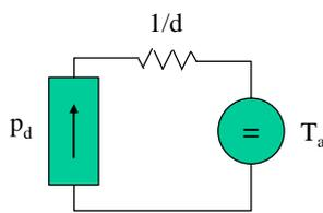
$$\left. \begin{aligned} \Delta T &= \frac{p_d}{d} \\ p_d &= Ri^2 \end{aligned} \right\} \Rightarrow \Delta T_{m\acute{a}x} = \frac{RI_{m\acute{a}x}^2}{d}$$
