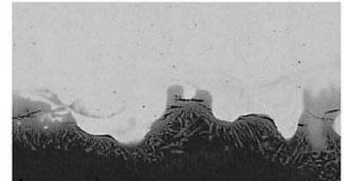
Cr 2 O 3 coating with a thickness of ca. 200 μm, deposited using a CO 2 laser and treated with a Nd-YAG laser.
