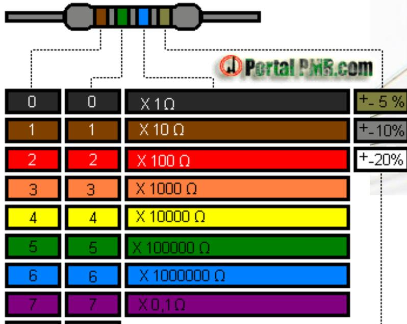
Diagram of a resistor with color bands and a table of color codes. The table lists the color code for each digit (0-9) and the multiplier for each band (0-7).
