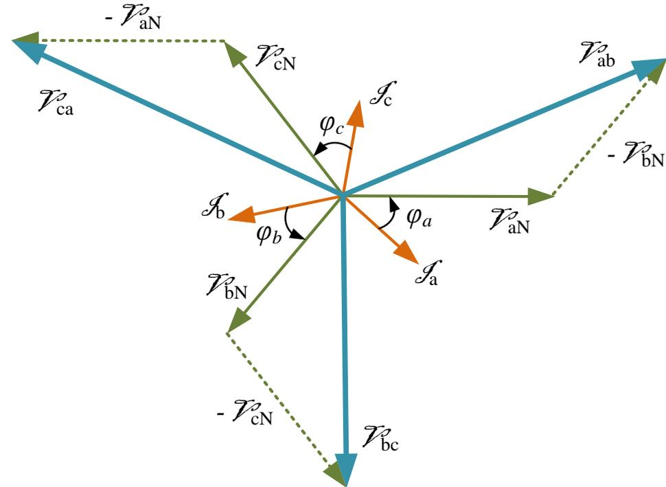
$$V_{ab}^p = V_{aN}^p (\sqrt{3} \angle 30^\circ)$$
