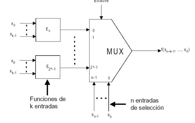
$$f(x_{n+k-1},...,x_n,x_{n-1},...,x_0) = f(z_{k-1},...,z_0,s_{n-1},...,s_0) = \sum_{i=0} E_i(z_{k-1},...,z_0) \cdot m_i(s_{n-1},...,s_0)$$
