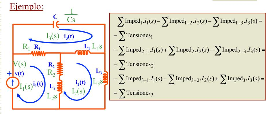
$$\begin{split} &(R_1+R_2+L_2.s).I_1(s)-(R_2+L_2.s).I_2(s)-R_1.I_3(s)=V\\ &-(R_2^{\binom{s}{2}}+L_2.s).I_1(s)+(R_2+L_1.s+L_2.s+L_3.s).I_2(s)-L_1.s.I_3(s)=0\\ &-R_1.I_1(s)-L_1.s.I_2(s)+(R_1+L_1.s+\frac{1}{C.s}).I_3(s)=0 \end{split}$$
