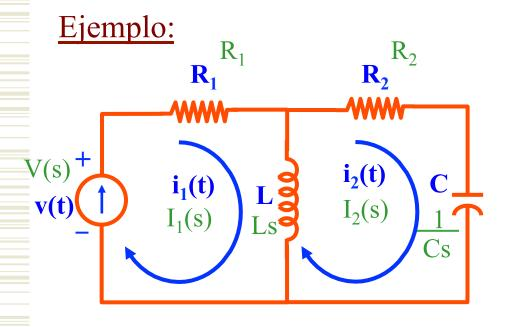
$$R_1.I_1(s) + L.s.I_1(s) - L.s.I_2(s) = V(s)$$
