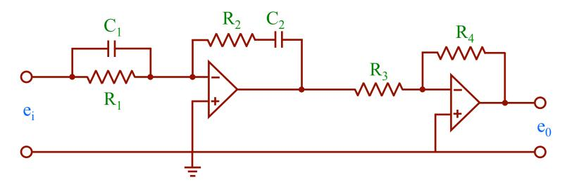
$$\frac{E_0(s)}{E_i(s)} = \begin{bmatrix} R_4.(R_1.C_1 + R_2.C_2) \\ R_3.R_1.C_2 \end{bmatrix} + \begin{bmatrix} R_4 \\ R_3.R_1.C_2.s \end{bmatrix} + \begin{bmatrix} R_4.R_2.C_1.s \\ R_3 \end{bmatrix}$$
