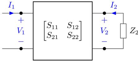
$$S_{11} = \frac{b_1}{a_1} \Big|_{a_2=0} = \frac{(V_1 - Z_1 I_1)/\sqrt{8Z_1}}{(V_1 + Z_1 I_1)/\sqrt{8Z_1}} = \frac{V_1 - Z_1 I_1}{V_1 + Z_1 I_1}$$
