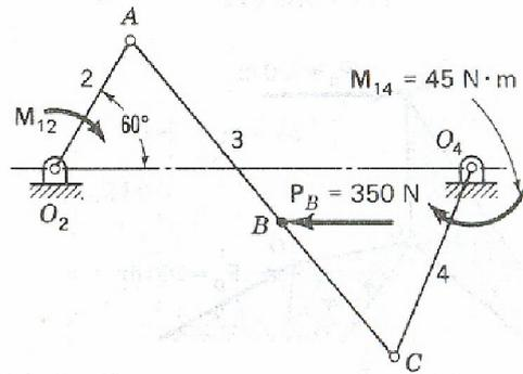
$$h_4 = 0,3 \text{ m}; \quad F'_{43} = \frac{45 \text{ N} \cdot \text{m}}{0,3 \text{ m}} = 150 \text{ N} = -F'_{23}; \quad F''_{23} = 330 \text{ N}; \quad F''_{43} = 180 \text{ N};$$
