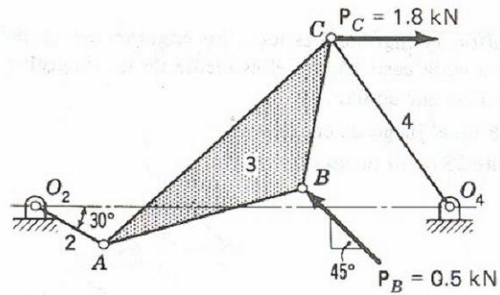
Datos:  $O_2A = 75 \text{ mm}$ ,  $AB = O_4C = 200 \text{ mm}$ ,  $AC = 300 \text{ mm}$ ,  $BC = 150 \text{ mm}$ ,  $O_2O_4 = 400 \text{ mm}$ .
