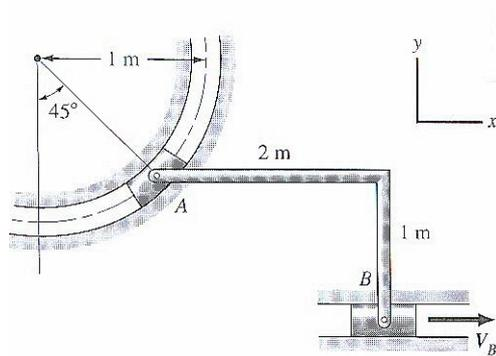
$$\vec{v}_A = \vec{v}_B + \vec{v}_{AB} = \vec{v}_B + \omega_{AB} \times \vec{R}_{AB} = 5 \cdot \dot{i} + \begin{vmatrix} \dot{i} & \dot{j} & \vec{k} \\ 0 & 0 & \omega_{AB} \\ -2 & 1 & 0 \end{vmatrix}$$
