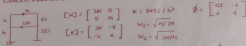
$$[M] = \begin{bmatrix} 2m & 0 \\ 0 & m \end{bmatrix} \quad K = 24EI/h^3 \quad \phi = \begin{bmatrix} 1/2 & -1 \\ 1 & 1 \end{bmatrix}$$
