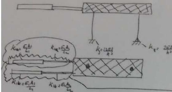
$$\frac{1}{k_{eq}} = \frac{1}{\frac{EI}{L_1}} + \frac{1}{\frac{EI}{L_2}} = \frac{\frac{EI}{L_1} + \frac{EI}{L_2}}{\frac{EI}{L_1} \cdot \frac{EI}{L_2}} \Rightarrow k_{eq} = \frac{EI \cdot EI \cdot L_1 \cdot L_2}{L_1 \cdot L_2 \cdot (EI \cdot L_1 + EI \cdot L_2)}$$
