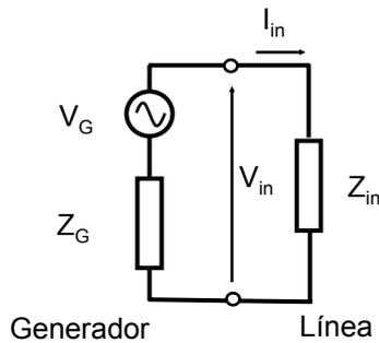
$$V_{in} = V_G \frac{Z_{in}}{Z_G + Z_{in}}$$
