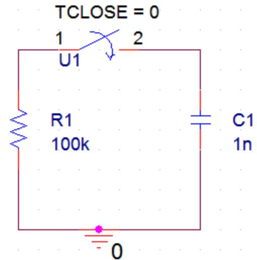
$$v(t) = v_0 e^{-\frac{1}{RC}(t-t_0)}$$
