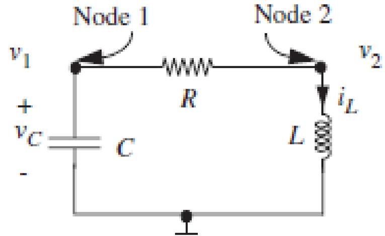
$$A \left( s^2 + \frac{R}{L} s + \frac{1}{LC} \right) e^{st} = 0 \Rightarrow \begin{cases} s_1 = -\frac{R}{2L} + \sqrt{\left(\frac{R}{2L}\right)^2 - \frac{1}{LC}} \\ s_2 = -\frac{R}{2L} - \sqrt{\left(\frac{R}{2L}\right)^2 - \frac{1}{LC}} \end{cases}$$
