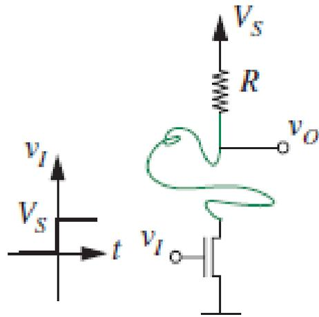
(a) Inverter with a long wire connecting the output and the MOSFET drain
