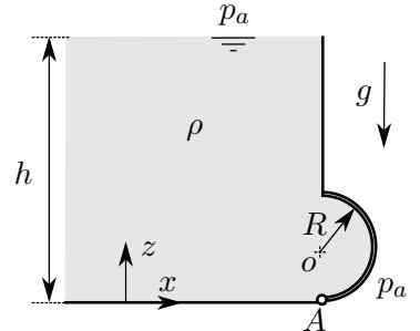
$$\text{Sol. a)} \quad \bar{F} = \rho g \pi R^2 (h - R) \bar{e}_x - \frac{2}{3} \rho g \pi R^3 \bar{e}_z, \quad \bar{M} = \rho g \pi R^3 (h - R) \bar{e}_y$$
