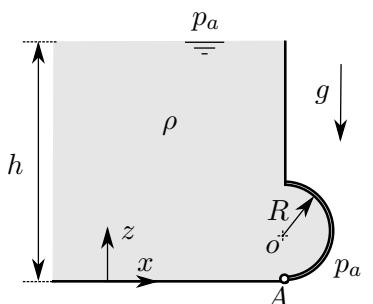
$$\text{Sol. a)} \quad \bar{F} = \rho g R b \left( 2(h-R) \bar{e}_x - \frac{\pi R}{2} \bar{e}_z \right), \quad \bar{M} = 2\rho g R^2 b (h-R) \bar{e}_y$$
