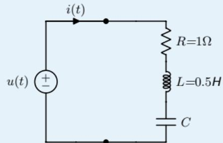
Hint: Active and apparent powers are  $S = \sqrt{\sum_k U_k^2} \sqrt{\sum_k I_k^2}$  and  $P = \sum_k U_k I_k \cos \phi_k$ , respectively. The reactive power, from Budeanu's definition, is  $Q = \sum_k U_k I_k \sin \phi_k$ .
