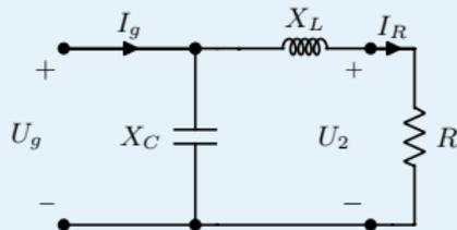
**CM2:** A bulb lamp with nominal values 150V, 1500W, is connected to a 250V power grid, in series with an inductive reactance such that the voltage across the lamp is 150V. Additionally, a capacitor is connected in parallel to achieve unitary power factor. Calculate:
