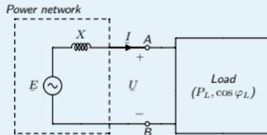
An electrical load is connected to a 230V power network.
