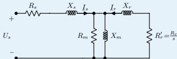
**CM56:** The circuit above represents an induction motor connected to a voltage source  $U_s = 220 \text{ V}$ , where  $s$  is the slip relating the current speed with the synchronous one. If the motor parameters are  $R_s = R_r = X_s = X_r = 1 \ \Omega$ ,  $R_m = 50 \ \Omega$  and  $X_m = 100 \ \Omega$ , find:
