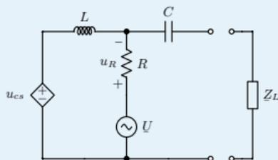
Find the value of impedance load,  $Z_L$ , for maximum average power transfer, and the average power delivered to the load.
