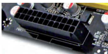
↑ Conector de corriente ATX12V 24p.
