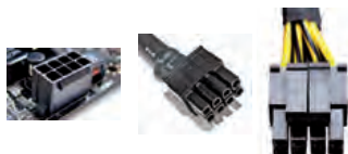
↑ Puerto y conectores EATX 12V.
