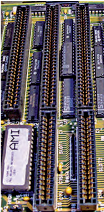
↑ Slots ISA (un slot XT y dos slots AT).
