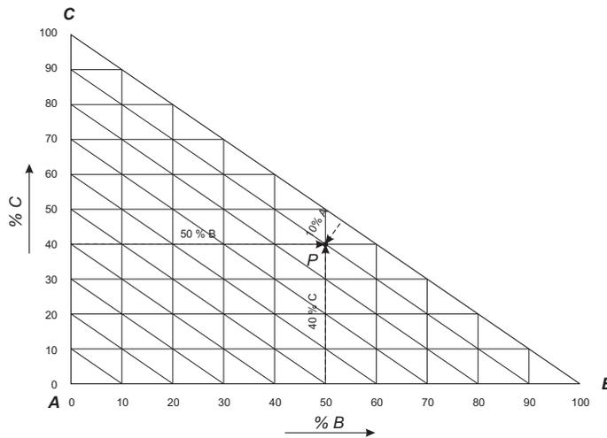
Figura A.3: Diagrama triangular rectangular
