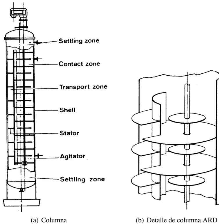
Figura 8.25: ARD («Asymmetric Rotating-Disk contactor»)
