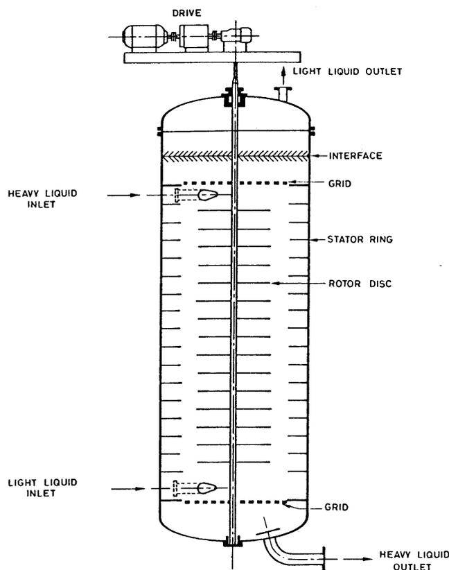
Figura 8.24: RDC (Rotating Disc Contactor)
